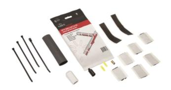
RAYCHEM WinterGard H910 Splice and Tee Kit is for use with WinterGard self-regulating heating cables to make splice, tee, and end seal connections. The kit contains materials for one splice and one end seal, or one tee connection and one end seal. This kit does not provide a power connection; use an H900 or H908 power connection kit for a complete installation.
