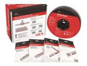
nVent RAYCHEM WinterGard Wet self-regulating trace heating cables provide energy efficient and easy to use solutions for pipe freeze protection and roof and gutter de-icing. This TruckPak kit includes heating cable, two H900 hardwired power/end seal kits, one H910 splice/tee kit, and one H903 application tape. Available as 120 V or 240 V, 100 ft, 6 W/ft.
