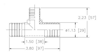
**Engineering Specification:** Zurn® 1-1/4" x 1-1/4" x 1" PEX barb tee. The QQT665X tee is used to transition a 1-1/4" main line to a 1" branch line.
