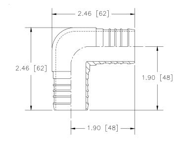
**Engineering Specification:** Zurn® 1-1/4" PEX barb elbow. The QQE66X elbow is used to make sharp 90° bends.
