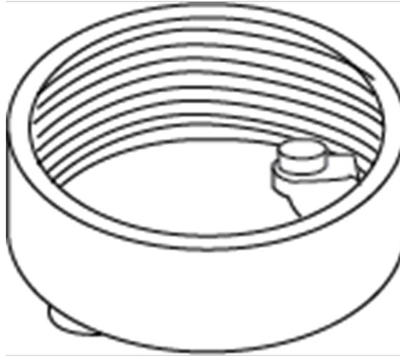
Installed either before or after concrete pour to create activation from duct. NOTE: Drill a 2 1/2" [64mm] hole in concrete and a 2 1/4" [57mm] hole in duct.
