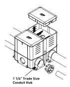
Box comes complete with reusable mudcap, insert spacer, conduit plugs and reducers. Reducers provided for reduction to 1 1/2", 1 1/4", 1", 3/4" and 1/2" [25mm, 19.1mm and 12.7mm] conduit. Minimum concrete depth is 4" [102mm] and maximum concrete depth is 6" [152mm]. Minimum capacity is 50 cu. in. [819mt] and maximum capacity is 100 cu. in. [1693mt]. Box dimensions are 4 1/8" W x 5 1/2" L x 6" H [105mm W x 140mm L x 152mm H].
