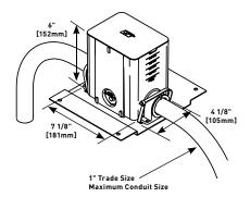
Box comes complete with reusable mudcap, insert spacer, conduit plugs and reducers. Reducers provided for reduction to 1", 3/4" and 1/2" [25mm, 19.1mm and 12.7mm] conduit. Minimum concrete depth is 3 1/2" [89mm] and maximum concrete depth is 6" [152mm]. Minimum capacity is 50 cu. in. [819mt] and maximum capacity is 100 cu. in. [1639mt]. Box dimensions are 4 1/8" W x 5 1/2" L x 6" D [105mm x 140mm x 152mm].
