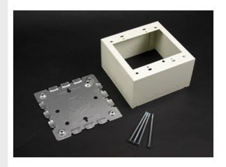
For deep devices such as momentary contact, remote control switches, and hospital signaling system devices. Base has 1/2" trade size KOs. Larger gang boxes available by special order. Two-gang: 4 3/4" L x 4 3/4" W [121mm x 121mm]. Accepts NEMA double-gang standard faceplates. NOTE: Certified to Canadian Safety Standards for sale in Canada. When ordering these products, change the "V" color prefix to "vc" or the "WH" color suffix to "WHC" to denote the Canadian versions.
