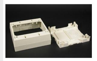
Two-gang. For deeper switches and devices. Base has rectangular KO to enable extension from existing flush wall box and 1/2" and 1" trade size concentric KOs. Accepts industry standard faceplates for switch and communication devices.
