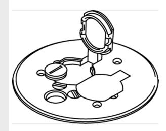
Supplied with 1/2" [12.7mm] screw plug for accessing communication cables. 5 1/2" [140mm] diameter for carpet applications only. Used in conjunction with the 881DIV to complete the dual service 881 PVC Floor Box. NOTE: For carpet or tile installations. All cover plates are furnished with gasket and three screws. The 895P Polycarbonate Series Cover Plates must be field modified for dual service.
