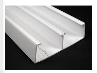
Two equal compartments - Base accepts single or Twin Snap Cover. 5400 Series raceway is available in 8' [2.4m] lengths with pre-punched mounting holes, packed 48' [14.6m] per carton.
