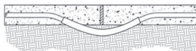
For cut expansion joints, dip the tubing below the slab to a safe distance at the cut lines
