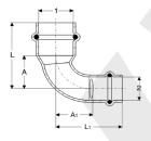
Viega ProPress 90° Reducing Elbow Copper P x P - Model 2916.3
