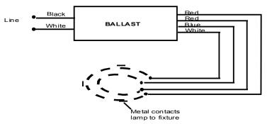
Ballast must be grounded. Install in accordance with National Electric Code.
