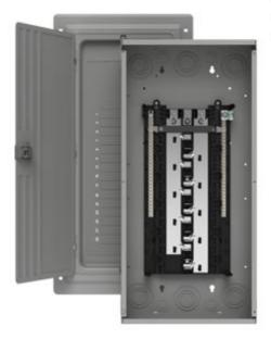
Siemens Low Voltage Residential Load Centers ES 3-Phase Indoor 150-225a Main Lug > 42 Circuits. Load Centers Type: 1Application: Residential V. Rating: 120/240V A. Rating: 200A phase: 3PH Load Regulation: 200A Wiring Conf: 3/4w Bus Rating: 200A Interrupt Rating: 22000AIC
