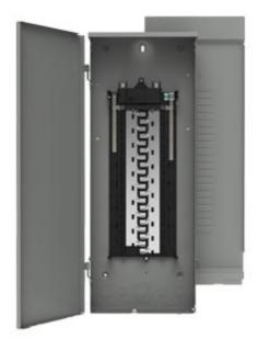
Siemens Low Voltage Residential Load Centers ES Single Phase Outdoor 150-225a Main Breaker 30-42 Circuits Load Centers 3070.9375 for residential applications. Rated 120/240V (200A).Overload, short circuit protection by integrated circuit breaker. (AIR 22000AIC). Outdoor Type 3R enclosure with surface mounting. No special features listed.
