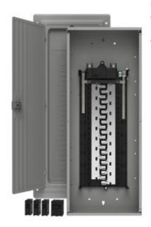
Siemens Low Voltage Residential Load Centers ES Single Phase Value Packs Main Breaker Load Centers 3214.6875 Type 1 for residential applications. Rated 120/240V (200A).Overload, short circuit protection by integrated circuit breaker. (AIR 22000AIC). Indoor Type 1 enclosure with combination mounting. No special features listed.
