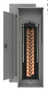
SIEMENS LOW VOLTAGE PL SERIES LOAD CENTER. FACTORY INSTALLED MAIN BREAKER WITH 54 1-INCH SPACES ALLOWING MAX 70 CIRCUITS. 1-PHASE 3-WIRE SYSTEM RATED 120/240V (225A) 22KA INTERRUPT. SPECIAL FEATURES: COPPER BUS, INTERCHANGEABLE MAIN, GRAY TRIM, NEMA TYPE1 ENCLOSURE FOR INDOOR USE.
