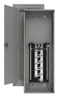
SIEMENS LOW VOLTAGE PL SERIES LOAD CENTER. MAIN LUG WITH 30 1-INCH SPACES ALLOWING MAX 54 CIRCUITS. 3-PHASE 4-WIRE SYSTEM RATED 120/240V OR 120/208V (200A) 100KA INTERRUPT. SPECIAL FEATURES: COPPER BUS, INTERCHANGEABLE MAIN, GRAY TRIM, NEMA TYPE1 ENCLOSURE FOR INDOOR USE.
