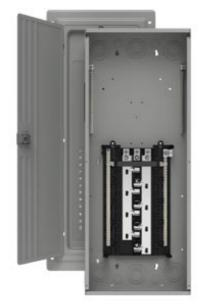
SIEMENS LOW VOLTAGE PL SERIES LOAD CENTER. MAIN LUG WITH 24 1-INCH SPACES ALLOWING MAX 42 CIRCUITS. 3-PHASE 4-WIRE SYSTEM RATED 120/240V OR 120/208V (200A) 100KA INTERRUPT. SPECIAL FEATURES: COPPER BUS, INTERCHANGEABLE MAIN, GRAY TRIM, NEMA TYPE1 ENCLOSURE FOR INDOOR USE.
