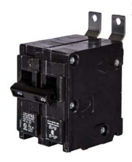
Siemens Low Voltage Molded Case Circuit Breakers Panelboard Mounting 240V Circuit Breakers - Type BL, 2-Pole, 120/240VAC are Circuit Protection Molded Case Circuit Breakers. Type: BL Application: Electrical Distribution Standard: UL 489 Voltage Rating: 120/240V Amperage Rating: 35A Trip Range: Thermal Magnetic Interrupt Rating: 10 AIC Number Of Poles: 2P
