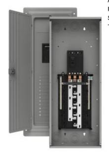
SIEMENS LOW VOLTAGE ES SERIES LOAD CENTER. FACTORY INSTALLED MAIN BREAKER WITH 24 1-INCH SPACES ALLOWING MAX 42 CIRCUITS. 3-PHASE 4-WIRE SYSTEM RATED 120/240V OR 120/208V (150A) 10KA INTERRUPT. SPECIAL FEATURES: ALUMINUM BUS, GRAY TRIM, NEMA TYPE1 ENCLOSURE FOR INDOOR USE.
