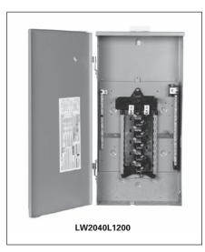
Load centers on this page through 225 amp feature a split neutral insulated bars. For service entrance applications, install bonding strap, and use both bars for neutral and ground conductors. For non service entrance applications, do not install bonding strap and use insulated bars for neutral conductors and bonded bar for ground conductors.
