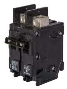
Siemens Low Voltage Molded Case Circuit Breakers General Purpose MCCBs - Type BQ, 2-Pole, 120/240VAC are Circuit Protection Molded Case Circuit Breakers. 2-Pole Common-Trip circuit breaker type BQ. Rated 120/240V (030A) (AIR 10 kA). Special features: Load side lugs are included.
