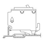
5. Push top of retainer back flush with face of breaker. Tail of retainer will snap out from in between the breaker poles and lock the breaker in place.
