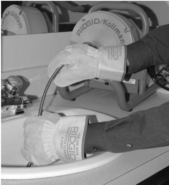
Figure 11 – Manually Feeding Cable
