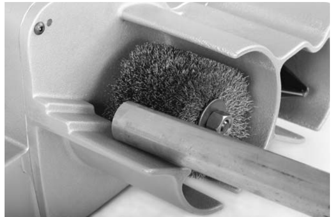
Figure 11 – Cleaning Tube O.D.
