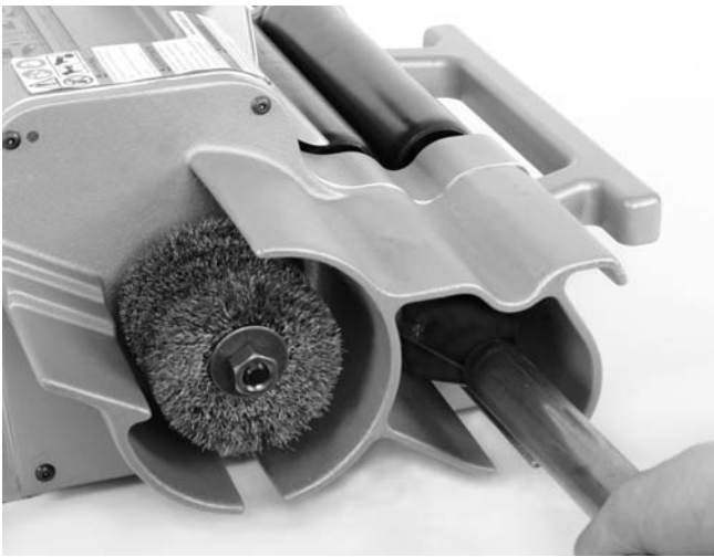
Figure 13 – Reaming I.D. of Tube
