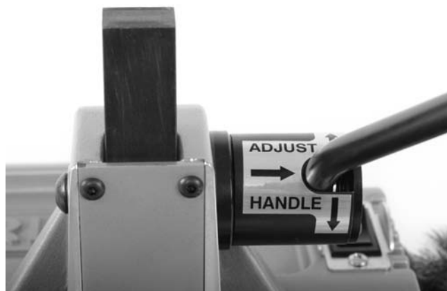
Figure 8 – Adjusting Handle Position
