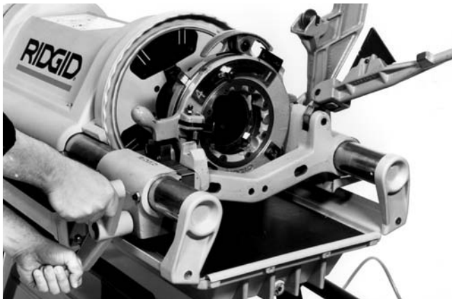
Figure 14 – Threading NPT/BSPT Threads with No. 714 or 914 Die Head
