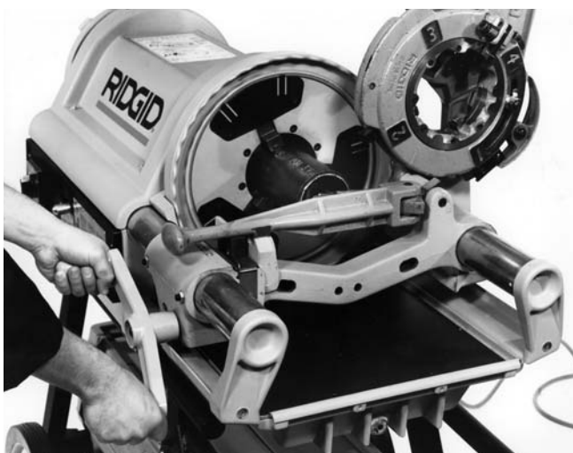
Figure 6 – Reaming Pipe with No. 744 Reamer
