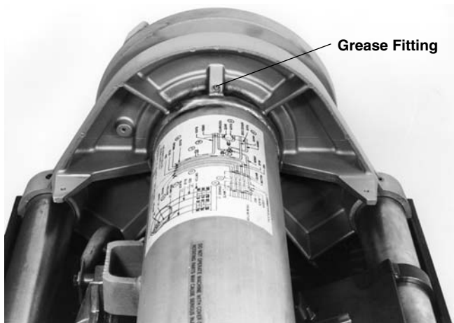
Figure 24 – Greasing Main Shaft Bearings
