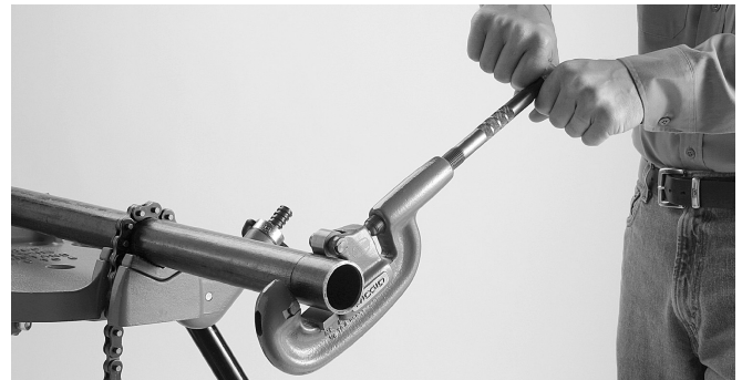
Figure 3 – Cutting End Of Pipe
