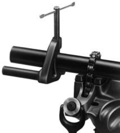
Figure 3 – Using No. 601 Support Arm when threading \frac{3}{4} " pipe and larger
