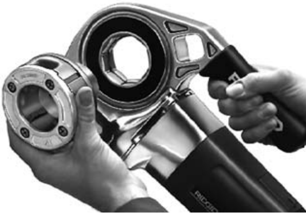
Figure 2 – Installing No. 11-R Drop Head Die Head
