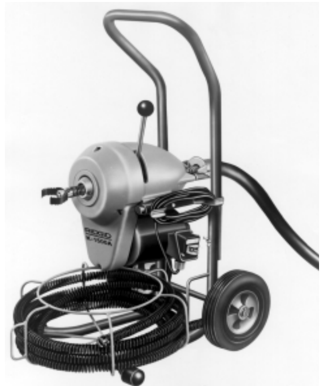
Figure 11 – Storing Cables On “A” Frame Models
