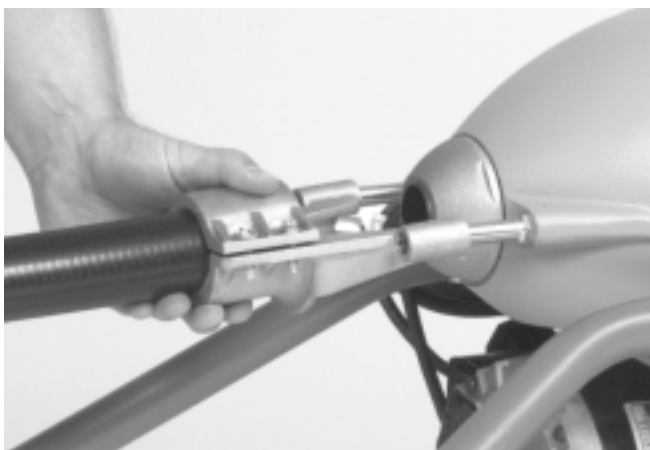
Figure 3 – Rear Guide Hose Attachment
