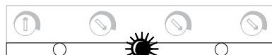
Middle LED on steady is Manual Override Mode Middle LED blinking is Evening Timer Mode
