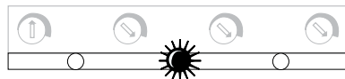
Middle LED on steady is Manual Override Mode Middle LED blinking is Evening Timer Mode
