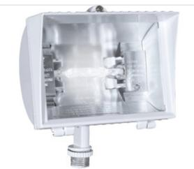
The Mini Curve. High quality die cast flood with rounded back and integral glare shield. Tempered glass lens. Gold plated socket contacts and 250°C Teflon coated wires for extended lamp life. 150 Watt double ended 130 volt Quartz halogen lamp supplied.
