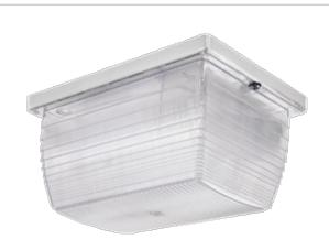
Compact ceiling mount fixture: 7, 9, 13, or 14 Watt fluorescent. Reflector is die-formed heavy gauge steel in white finish with clear vandalproof polycarbonate refractor. Lamp supplied.
