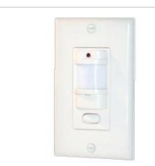
Fits decorator wall plates with only 1/2" protrusion. 120 volts. Gangable. Full 180° view covers 1000 sq. ft Works with electronic ballasts. Can be wired in parallel. LED indicator, wallplate included. Can also be used as a ceiling sensor. Must have hot and wires in box.
