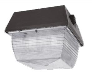
Medium size ceiling mount fixture: 35, 50 and 70 Watt HPS, 50 and 70 Watt Metal Halide. Housing is die cast aluminum with clear vandalproof polycarbonate refractor. Quartz Restrike models available. Lamps supplied.
