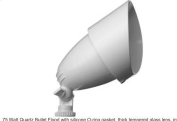
75 Watt Quartz Bullet Flood with silicone O-ring gasket, thick tempered glass lens, internal and external cooling fins. Gold plated socket contacts and 250°C Teflon coated wires for extended lamp life. Lamp supplied.
