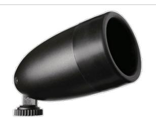
Premium PAR38 Flood with large, molded high temperature black silicone gasket that totally seals lamp. Die cast aluminum housing. EZ Locknut. Suitable for mounting within 4' of the ground. PAR38 or PAR20, 150 Watt max. Lamp not supplied.
