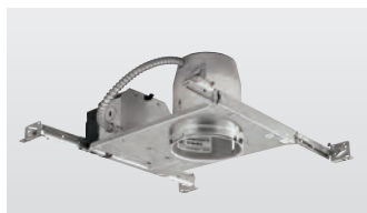
P816-TG Ceiling opening: 4-1/2" Plaster frame: 7-7/8" x 10-3/4" Recessed depth: 5-1/2" Pryouts: 1/2" & 3/4"
