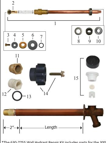
\*The 630-7755 Wall Hydrant Repair Kit includes parts for the 300, 400 and 500 Series hydrants, some of which are not pictured here. When repairing a hydrant you will have parts left over.
