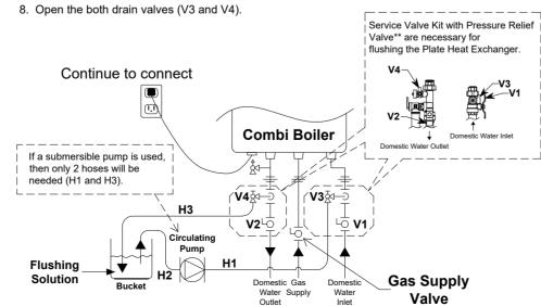
\*\* Service Valve Kit with Pressure Relief Valve may be purchased as an accessory from an authorized wholesaler. They allow for full diagnostic testing and easy flushing of the system. Refer to appliance's installation manual or reach out to our customer care, if more information is needed for flushing. Contact details are available on the rating plate of the appliance.
