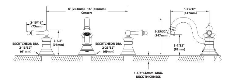
NOTE: FOR DECK THICKNESS 1-3/8" - 3", USE SERVICE KIT #115001. VALVES INSTALL THROUGH 1-1/4" DIA. HOLE
