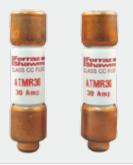
Amp-Trap® ATMR fuses, in the Class CC family, are the smallest dimension 600VAC/DC fuses suitable for branch circuit protection. The ATMR is a popular choice for economical protection of control circuits and control circuit transformers where available short circuit currents exceed 10,000 amperes. ATMR's rejection dimensions prevent substitution by lesser rated fuses. These fast acting fuses give currentlimiting protection to general circuits.
