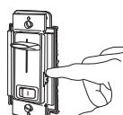
**Note:** If knob has little effect on fan speed, reset minimum speed.
