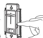
**Note:** If knob has little effect on fan speed, reset minimum speed.
