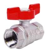
Maintenance-free, dual Viton® O-ring stem design, light weight and durable forged traditional brass body, blow-out proof stem, PTFE seats for improved wear. Chrome plated forged brass. Coated cast aluminum tee handle that is lightweight and compact in size. Available in sizes and configurations 1/2"- 1", FNPT x FNPT.
