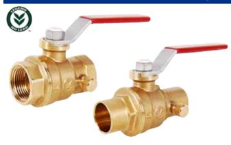
Maintenance-free, dual Viton® O-ring stem design, light weight and durable forged no lead brass body, blow-out proof stem, PTFE seats for improved wear. Ball with drain for maintenance or to prevent freeze. Dacromet® coated steel handle and nut for greater corrosion resistance. Constructed of no lead binary brass alloy. Suitable for potable water applications. Available in sizes and configurations 1/2"- 1", FNPT x FNPT and 1/2"- 1", Sweat x Sweat.
