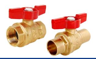
Maintenance-free, dual Viton® 0-ring stem design, lighter weight and durable forged traditional brass body, blow-out proof stem, PTFE seats for improved wear. Coated cast aluminum tee handle that is light weight and compact in size. Available in sizes and configurations 1/2" x 1", FNPT x FNPT and 1/2"-1", Sweat x Sweat.
