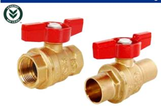
Maintenance-free, dual Viton® 0-ring stem design, lighter weight and durable forged no lead brass body, blow-out proof stem, PTFE seats for improved wear. Coated cast aluminum tee handle that is light weight and compact in size. Available in sizes and configurations 1/2" x 1", FNPT x FNPT and 1/2"-1", Sweat x Sweat.
