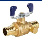
Maintenance-free dual EPDM® O-ring stem seal, zinc plated steel tee handle, CWP 400 PSI, with drain. Third Party certified no lead ANSI/NSF 61-G & DZR ANSI/NSF 14, IAPMO. ASTM F1806. Configuration and Sizes: PEX x PEX, 1/2"-1".
