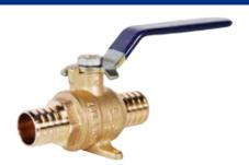
Maintenance-free dual EPDM® 0-ring stem seal, zinc plated steel handle with vinyl sleeve and drop ears. CWP 400 PSI. Third Party certified no lead ANSI/NSF 61-G & DZR ANSI/NSF 14, IAPMO. ASTM F1806. Configuration and Sizes: PEX x PEX, 1/2"-1".
