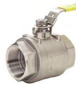
2-Piece Full Port 316 Stainless Steel Body, Ball & Stem 304 Stainless Steel Handle & Nut
