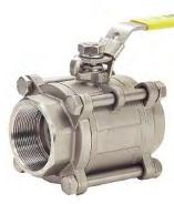
3-Piece Full Port 4-Bolt 316 Stainless Steel Body, Ball & Stem 304 Stainless Steel Handle & Nut
