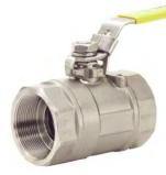
2-Piece Large Port 316 Stainless Steel Body, Ball & Stem 304 Stainless Steel Handle & Nut
